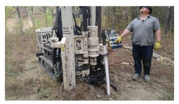
11-08-2016-003: The geoprobe was used to help remove the casings and over drill the well if the casing broke during removal.
